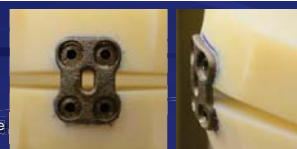
Prototype Magnetic Plate and Screws for Testing
