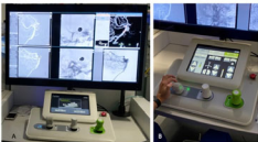
Figure 3 The operator's perspective. (A) The screen and the control console. The robotic arm is operated using three joysticks: one for microcatheter, one for microwire and one for the device (stent and coil). (B) Closer view of the control console showing the screen during coil placement. The small screen shows three columns, each corresponding to a joystick, with additional commands such as millimetric moves for the microcatheter and devices or predefined rotations for the microwires.
